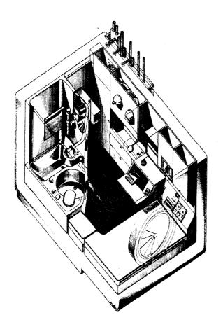
Fig. 7. Kisho Kurokawa, Nagakin Capsule Tower, Tokyo, 1972. Detail isometric of prefabricated capsule dwelling.
